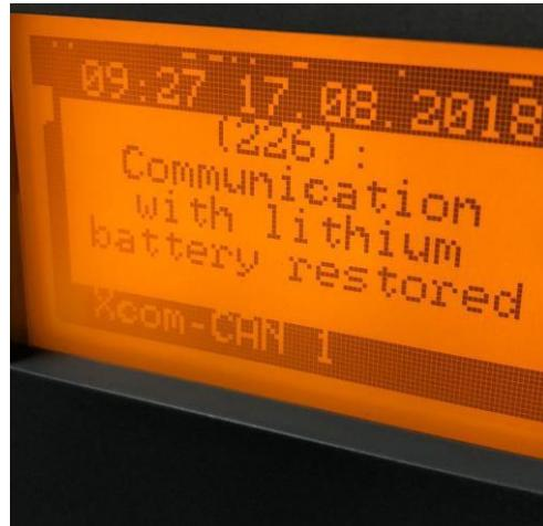
Once the communication is correct try to disconnect the CAN cable from the battery to the X-Com, must show a RED BACKGROUND
